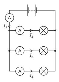
The currents measured by the ammeters are shown.
